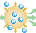
N moves out through the polymer coating as temperature increases
